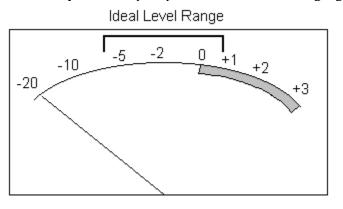
Don't worry too much about making sure the levels are exactly in the middle of the meter. You will find that if you set a given pot to the zero mark on the scale, the meter levels you will get will be acceptable. You will only have to adjust maybe one or two songs per show. There is compression equipment the station uses to smooth out the different levels of songs so that they are all the same to the audience. The meters only show your levels, not the levels of what is actually on the air.
